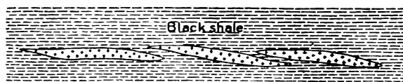
FIGURE 4.—Diagram showing the overlapping of lenticular porphyry sills in the black shales south of Copper Creek. Some of the lenses are 10 to 15 feet thick.
